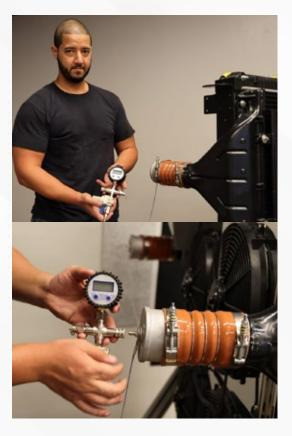
1. Once the pressure gauge is secured you can attach an air hose to begin the test.
